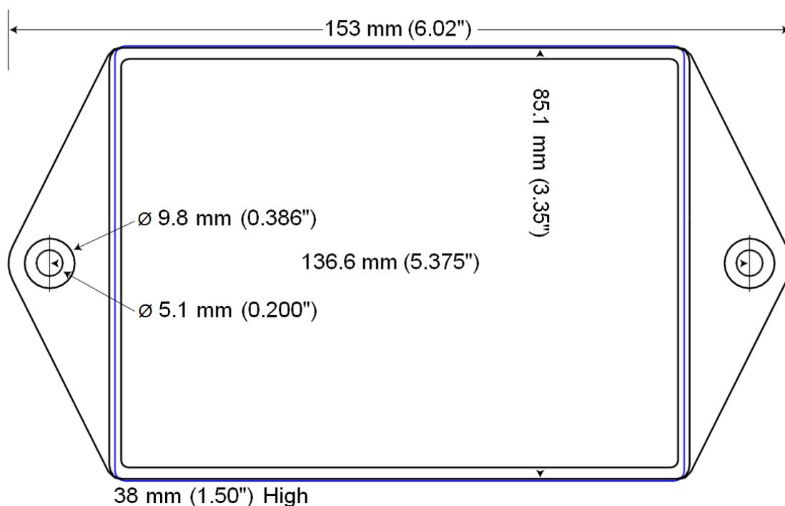
The meter has two mounting holes spaced 5.375 inches (137 mm) apart (center to center). These mounting holes are normally obscured by the detachable screw terminals. Remove the screw terminals by pulling outward while rocking from end to end. The meter may be used as a template to mark mounting hole positions, but do not drill the holes with the meter in the mounting position because the drill may damage the connectors and leave drill shavings in the connectors.
